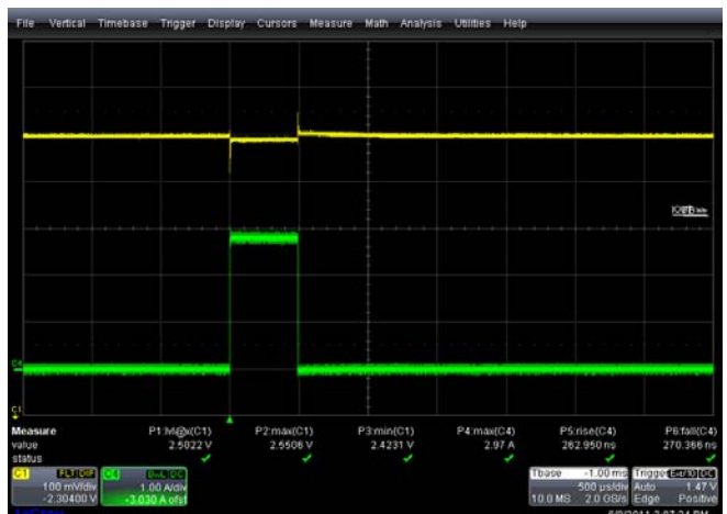
FIGURE 8. LOAD TRANSIENT, V_{IN} = 3.3V , V_{OUT} = 2.5V , C_{OUT} = 220\mu F 25mΩ
