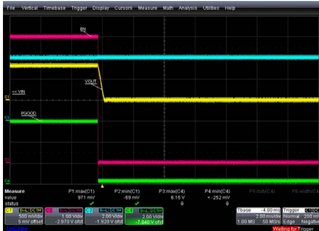
FIGURE 5. SHUTDOWN WAVEFORM: V_{IN} = 6.0V , V_{OUT} = 0.8V , EN HIGH TO LOW
